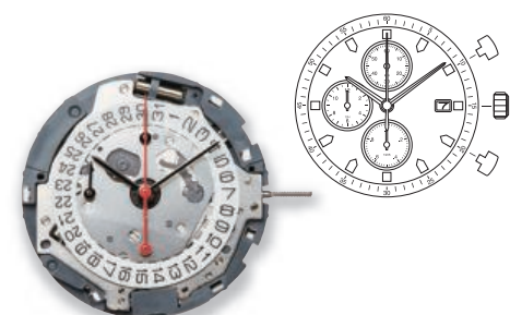
OS60 Height 4.13mm Chrono hour / min / sec, 1/20 second 2 years battery life (SR927W)
