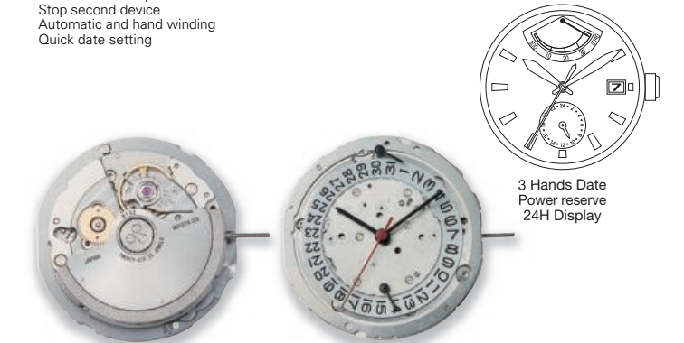
9132 Height 5.52mm / 26 Jewels 28800 vibrations per hour Stop second device Automatic and hand winding Quick date setting
