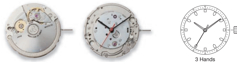
9039 Height 3.90mm / 24 Jewels 28800 vibrations per hour Stop second device Automatic and hand winding
