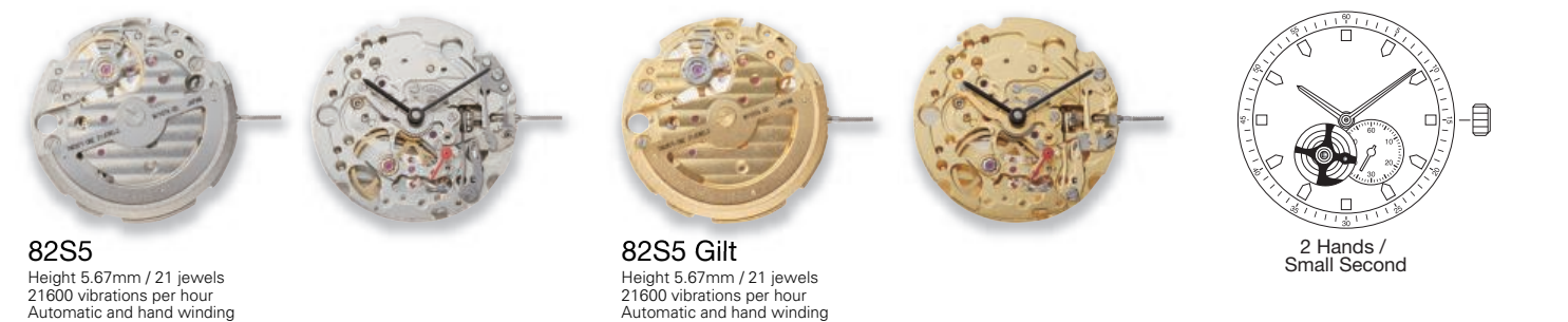
82S0 Height 5.67mm / 21 jewels 21600 vibrations per hour Automatic and hand winding
