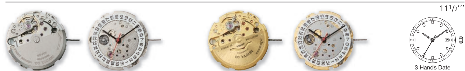
8215 Height 5.67mm / 21 jewels 21600 vibrations per hour Automatic and hand winding Quick date setting
