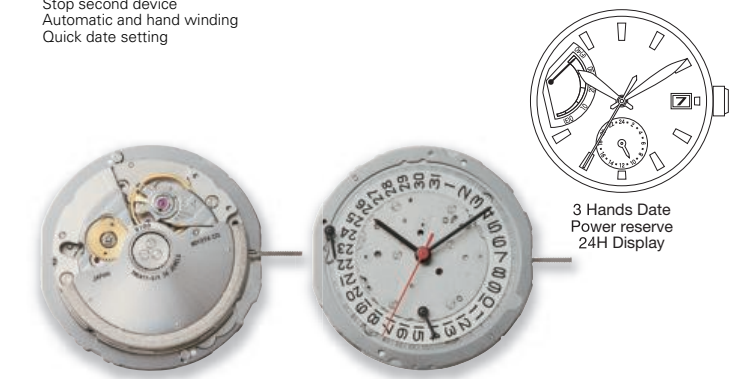
9134 Height 5.52mm / 26 Jewels 28800 vibrations per hour Stop second device Automatic and hand winding Quick date setting
