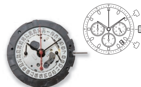
OS25 Height 5.10mm Chrono min / sec, 1/20 second, 24 hour 2 years battery life (SR927W)
