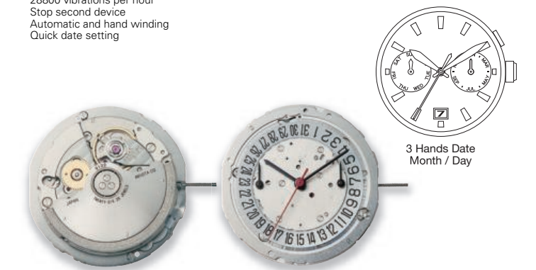
9122 Height 5.52mm / 26 Jewels 28800 vibrations per hour Stop second device Automatic and hand winding Quick date setting
