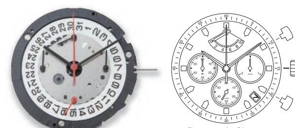
6SA2 Height 4.90mm Chrono hour / min / sec, 1/20 second 4 years battery life (SR927W)
