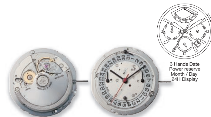
9100 Height 5.52mm / 26 Jewels 28800 vibrations per hour Stop second device Automatic and hand winding Quick date setting
