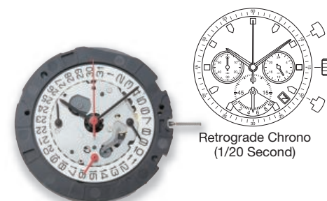
OS22 Height 5.10mm Chrono min / sec, 1/20 second, 24 hour 2 years battery life (SR927W)
