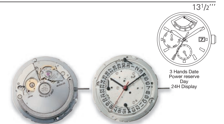
9110 Height 5.52mm / 26 Jewels 28800 vibrations per hour Stop second device Automatic and hand winding Quick date setting
