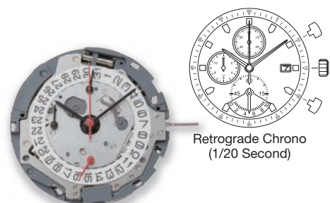
OS62 Height 4.13mm Chrono hour / min / sec, 1/20 second 2 years battery life (SR927W)
