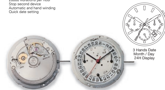
9120 Height 5.52mm / 26 Jewels 28800 vibrations per hour Stop second device Automatic and hand winding Quick date setting
