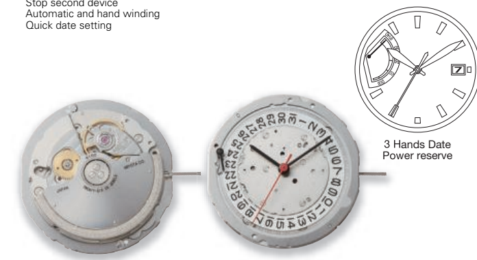
9133 Height 5.52mm / 26 Jewels 28800 vibrations per hour Stop second device Automatic and hand winding Quick date setting
