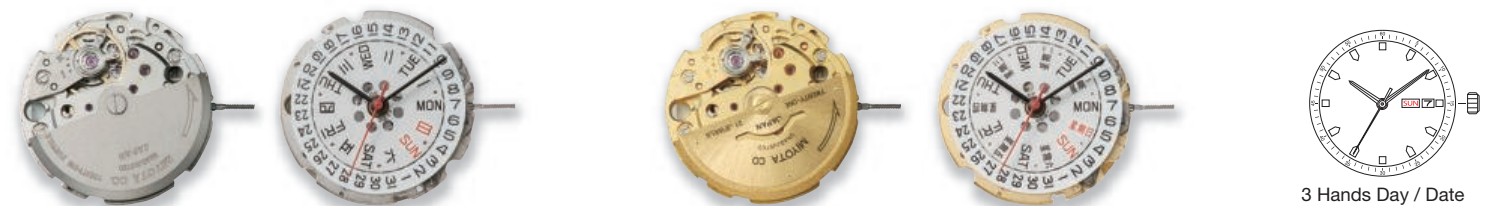
8205 Height 5.67mm / 21 jewels 21600 vibrations per hour Automatic and hand winding Quick day / date setting
